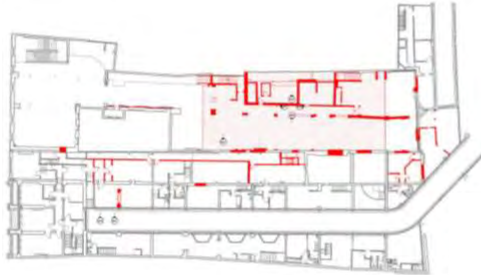
First Floor Demolition Plan
