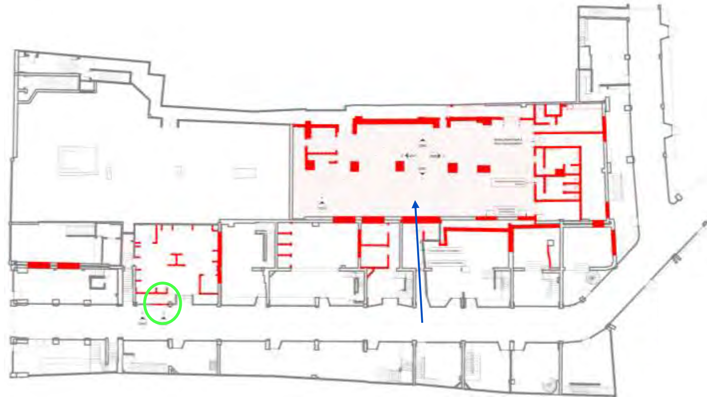
Ground Floor Demolition Plan
